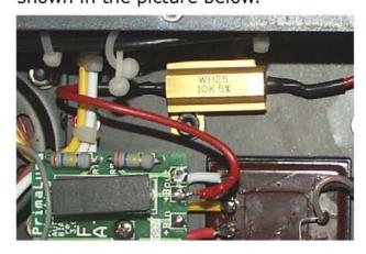
Put the screw back into its hole and tighten securely. Make sure the resistor is sitting flat against the chassis to ensure proper heat dissipation. When installed, the resistor will be positioned as shown in the picture on the left.
