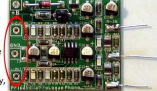
so be careful not to use too much solder. Just make sure it is enough to hold the wire securely to the board and does not form a solder bridge to other points nearby.
